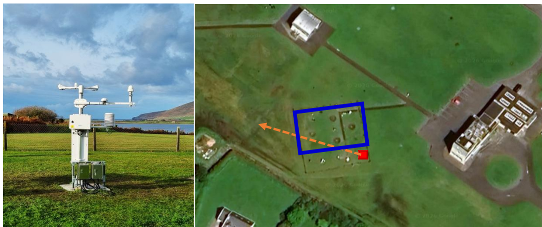
Figure 3. (left) The mount point of the FD70 sensor and of the RM60 sensor at Valentia Observatory. (right) the satellite map view of the test site, where the red symbol locates the mount point of the FD70 and the RM60 sensor, the orange arrow indicates the view of direction in the photo on the left. The blue rectangle indicates the area of pit mounted rain gauges of Valentia Observatory.
